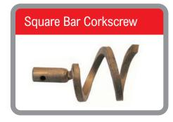
The best of all service tools with a protected cutting edge which operates as the tool is withdrawn, ripping apart difficult stoppages. Material: 10 x 10mm square bar- bright steel, cold rolled and welded to coupling - bright steel free cutting. (Hardened)
