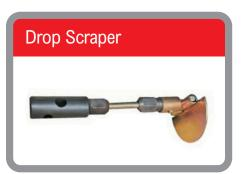
Designed to remain flat when pushed in and opens when pulled back. Used for sand and silt.
