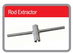
Locks to rods. When alternately turned sharply left and right is useful for getting through stubborn stoppages or pulling rods out of line. Material: Centre piece bright steel 25mm dia milled to accept 8mm steel rods. 12mm bright steel welded to centre.
