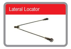
The Lateral / Branch locator is used for finding lost laterals or manholes. Two brass guide wheels are used to locate branch. By counting number of rods the distance can be measured.
