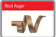
Cuts through roots, removes grease and removes sand, efficient when used with waterflow. Material: 20mm x 5mm spring steel flat bar, sharpened cutting edges, pointed front welded
